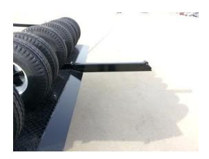
> Sliding rear lifting arm - No container jack needed - Simply lower or raise trailer bed to do the lifting
