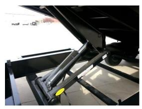
Power tilt scissors lift with dual purpose remote control
