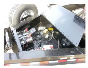
Double hinged utility box for easy access to hydraulics, batteries and electronics
